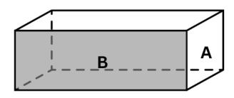
Let a represent the longest diagonal, b represent the diagonal of the base, c represent the diagonal of lateral face A, and d represent the diagonal of lateral face B.
